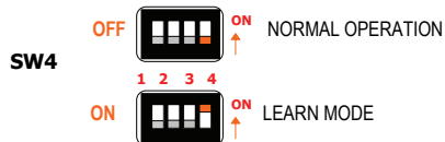
Figure 9: Dip Switch Configuration
