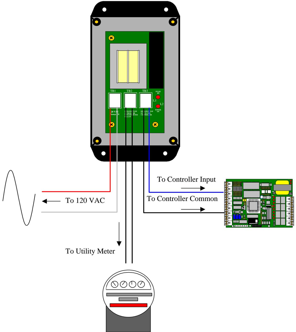
FIGURE 2: Wiring connections
