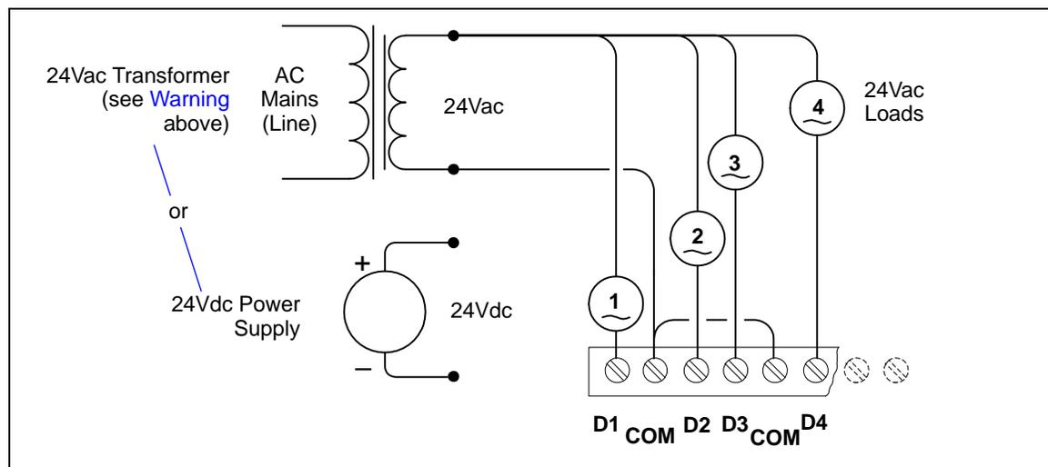
Note that the two common DO terminals are isolated from each other. This is useful if controlled loads are powered from different circuits.
